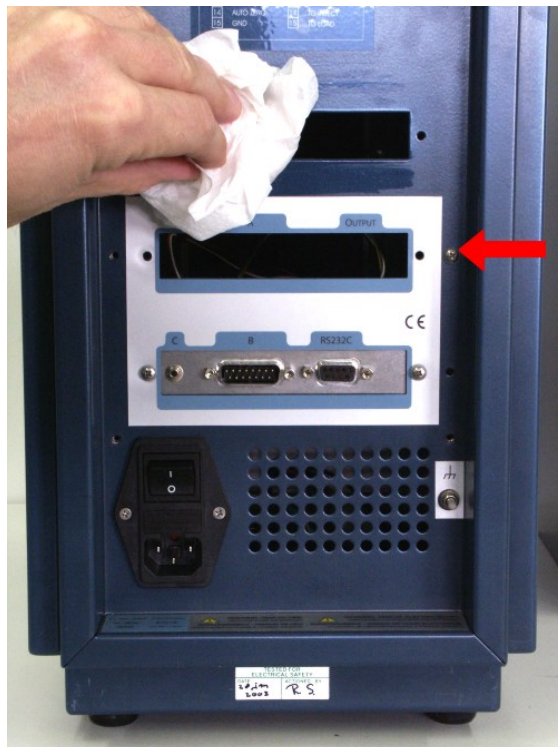
Figure 21 Degrease rear panel with ethyl alcohol.
