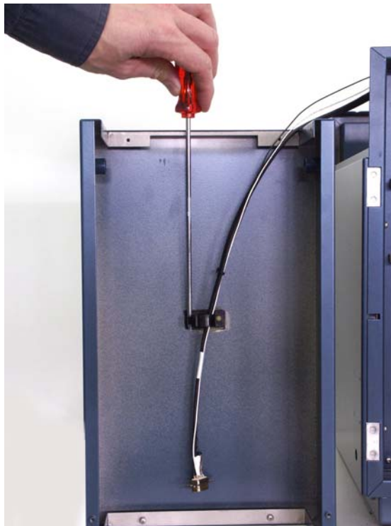
Figure 27 Release of cable clamp of the internal cell cable of sensor board 1.
