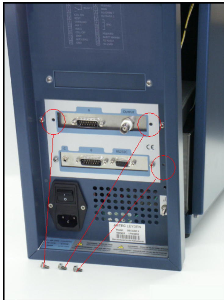
Figure 7 Removal of sensor board from the connector panel.
