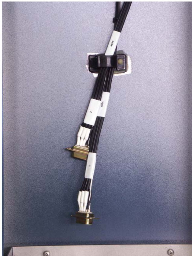
Figure 31 Both internal cell cables in black cable clamp on bottom side of DECADE II top-cover.
