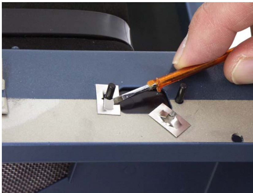
Figure 28 Clearing sub-D connector mounting position on oven compartment: removal of black cover.
