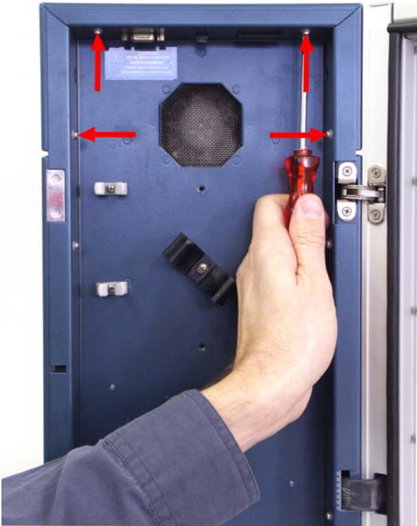
Figure 26 Removal of screws of top cover in oven compartment.
