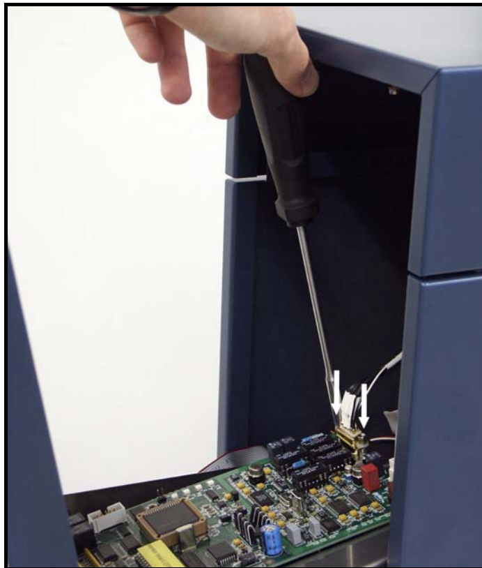
Figure 6 Removal of internal cell cable connector.
