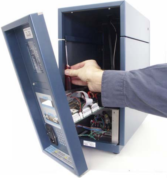
Figure 25 Removal of screws of top cover at back-side.
